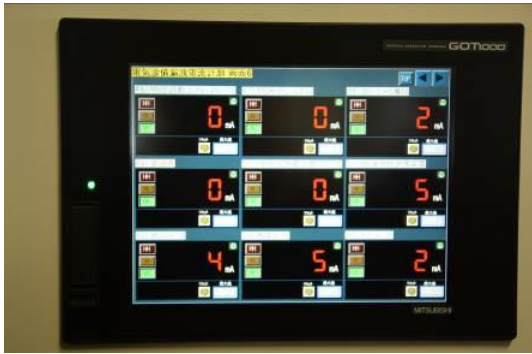
Pictures 8 and 9: Main display screen (Pic 8) and individual monitoring results display screen (Pic 9) on the GOT. Values exceeding the set threshold values light up in yellow or red.
